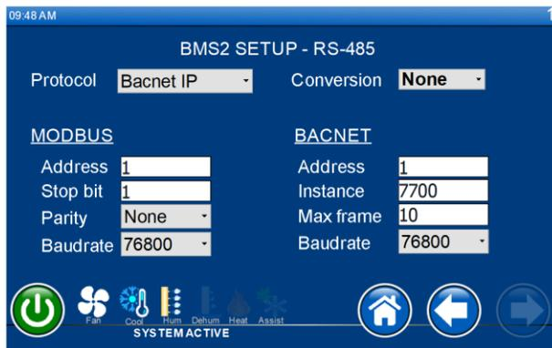
Figure 14. BMS2 (RS-485) setup
