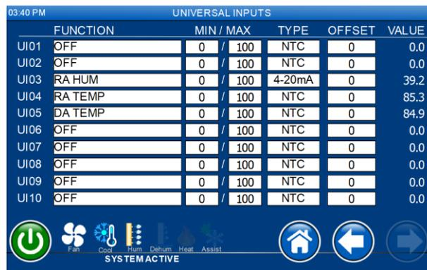
Figure 29. Factory setting analog inputs
