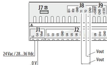
Figure 7 Analog outputs
