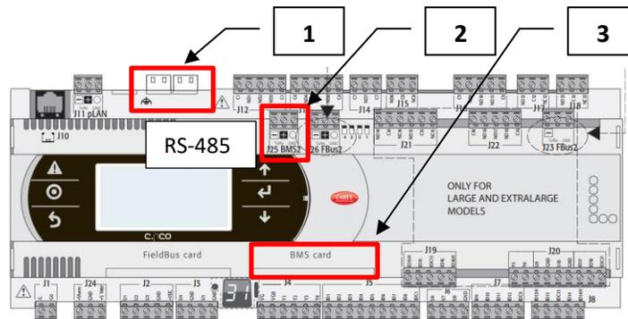
Figure 13. Communication ports
