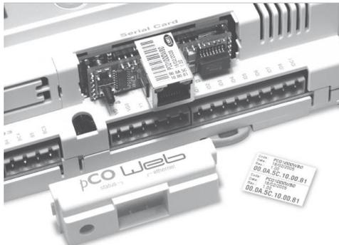
Figure 55 - Installing PCOWeb
