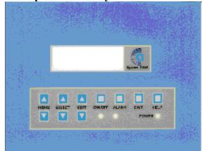
The *System 2200 xs* consists of a microprocessor controller located in the electrical panel of the Compu-aire unit, and the front panel mounted keypad/display microprocessor unit shown at left. In this manual, "controller" means the microprocessor board, "keypad" or "display" refers to the panel mounted unit shown at left.
