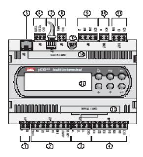
The *System 2200* main board is the core of the unit and will operate stand-alone without the need for the terminal unit. The main board is where all sensors and controlled devices are connected. The main parts are:
