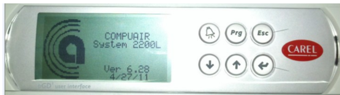
Figure 3 - Controller with built in Internal display
